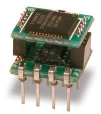
InfoChip is the technology that allows DMX devices without RDM capability to be recognized by InfoGate and communicate back to the system.
