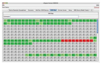
InfoGate software allows interactive, remote DMX addressing via drag & drop. In this instance, the red squares indicate overlapping DMX addresses.
