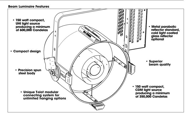
This compact, next generation beam projector uses the latest developments in optical and mechanical design, to give today's lighting designers another tool in their ever expanding arsenal of lighting effects. The BP-2 Beam Luminaire produces an extremely intense soft edge narrow 10°-13° beam (lamp dependent) of light several times more intense than an ordinary spotlight of similar wattage.
