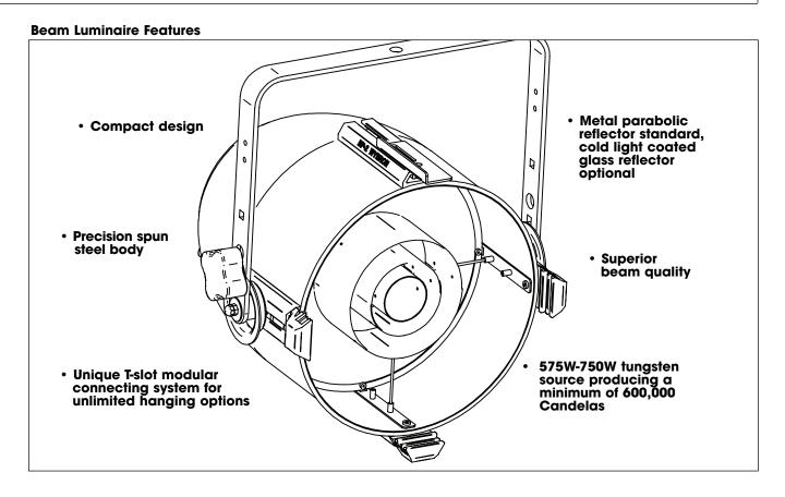
This compact, next generation beam projector uses the latest developments in optical and mechanical design, to give today's lighting designers another tool in their ever expanding arsenal of lighting effects. The BP-2 Beam Luminaire produces an extremely intense soft edge narrow  $10^\circ$  beam of light several times more intense than an ordinary spotlight of similar wattage.
